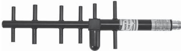
The Telewave ANT1920Y9-WR is a rugged, wideband, high gain Yagi antenna for the broadband PCS bands, designed for handheld use with many types of portable wireless analyzers. This antenna can also be installed for fixed use in any environment. The antenna uses six solid brass elements, and produces 9.3 dBd forward gain with excellent front-to-back performance. Construction and design are optimized to prevent RF intermodulation, and ensure precise pattern control.
