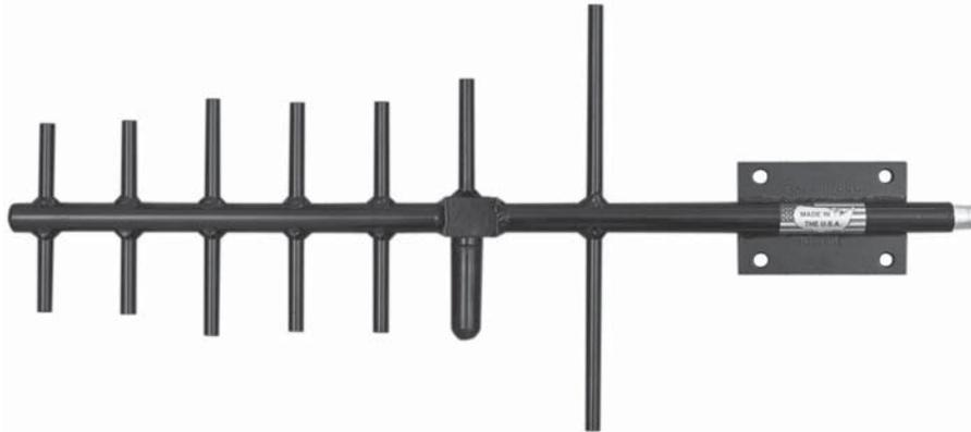
The Telewave ANT850Y10-WR is a high performance directional antenna, designed especially for point to point as well as point/multipoint applications. This antenna produces 10 dBd forward gain with an excellent front-to-back ratio. Solid aluminum elements with 360° welds prevent intermodulation and provide exceptional strength.
